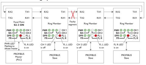
If an optical fibre segment fails, the ODW-710-F2 focal point will switch mode and start sending out data on both optical fibre ports, CH 1 and CH 2, simultaneously. Responses from the PROFIBUS slaves are sent back to the PROFIBUS master in the opposite direction, as normal. To determine witch fibre segment has failed, look at the FL L, CH 1 and CH 2 LED's as show in the picture above.
