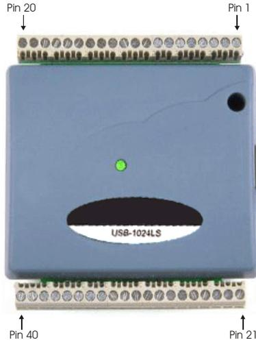
Figure 3-2. USB-1024LS screw terminal pin numbers
